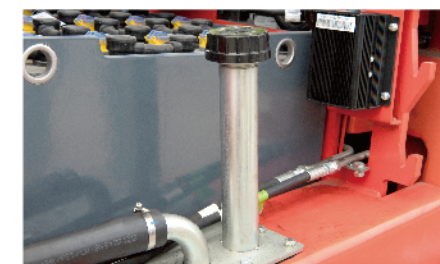
The hydraulic oil tank is located on the left side for easy filling and checking.
