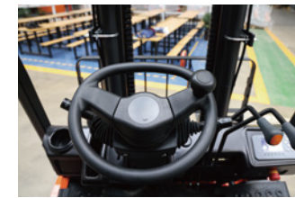
U design of steering wheel, front-located multi-way valve operating device makes the operation effortless and comfortable.
