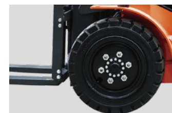
Big diameter tyres with better performance for outdoor application, and comfortable driving experience, optional to have solid tyres and non marking tyres.
