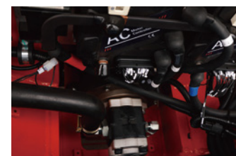
Lifting Motor located in high position so the truck can operate in areas where water may be present.
