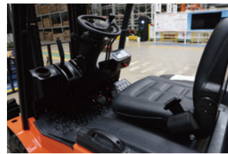
The seat can be adjusted back and forth so that the operator can choose the ideal driving position.
