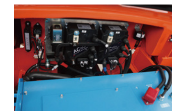
Controller assembly located on higher position for better ventilation and maintenance.
