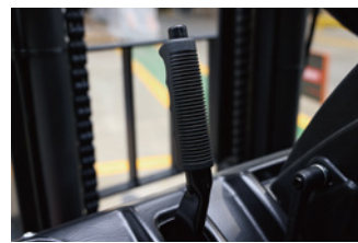
The truck has a long tiller ratchet parking brake design for easy operation.
