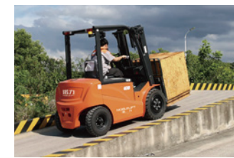
Ratchet-type parking brake allows the truck stop and hold at a slope of 15% without concern.
